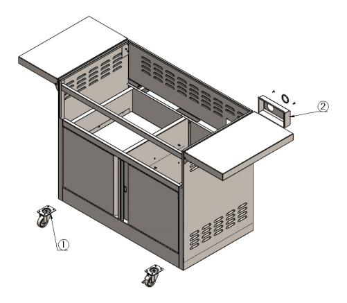
**STEP 1**: Two (2) people recommended for this assembly. Remove packaging and protective film from surface of cart (it is normal to see residue from protective film and recommended to wipe down cart with stainless steel cleaner once removed).
